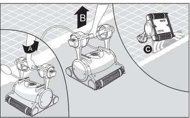
Using the floating cable, bring the Pool Cleaner to the pool's edge. Using the handle remove the Pool Cleaner from the pool.
