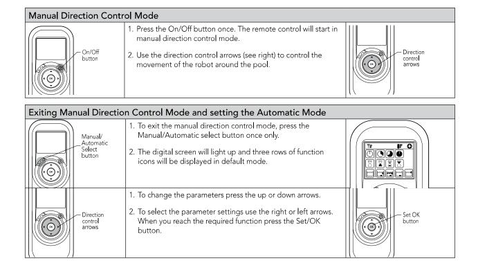
Press the Manual/Automatic select button and then choose the desired parameters according to the following table:
