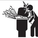
**HAZARDOUS PRESSURE: STAND CLEAR OF PUMP AND FILTER DURING START UP**
